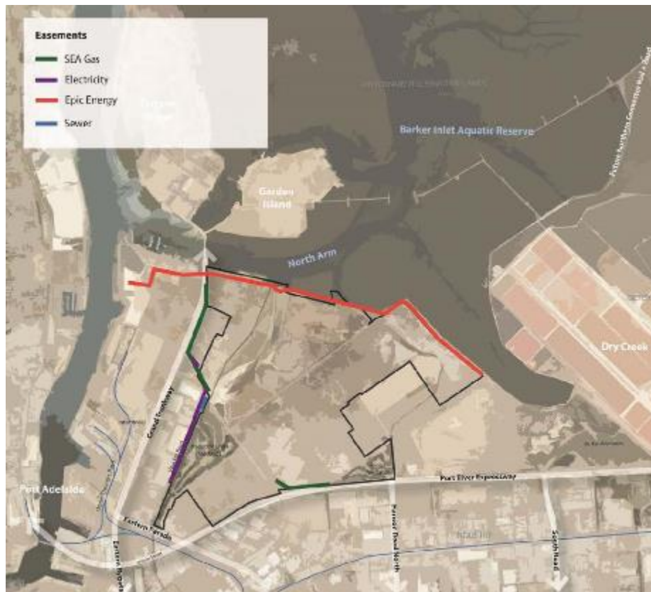
FIGURE 4-2: EASEMENTS IN MAGAZINE CREEK AND RANGE WETLAND
