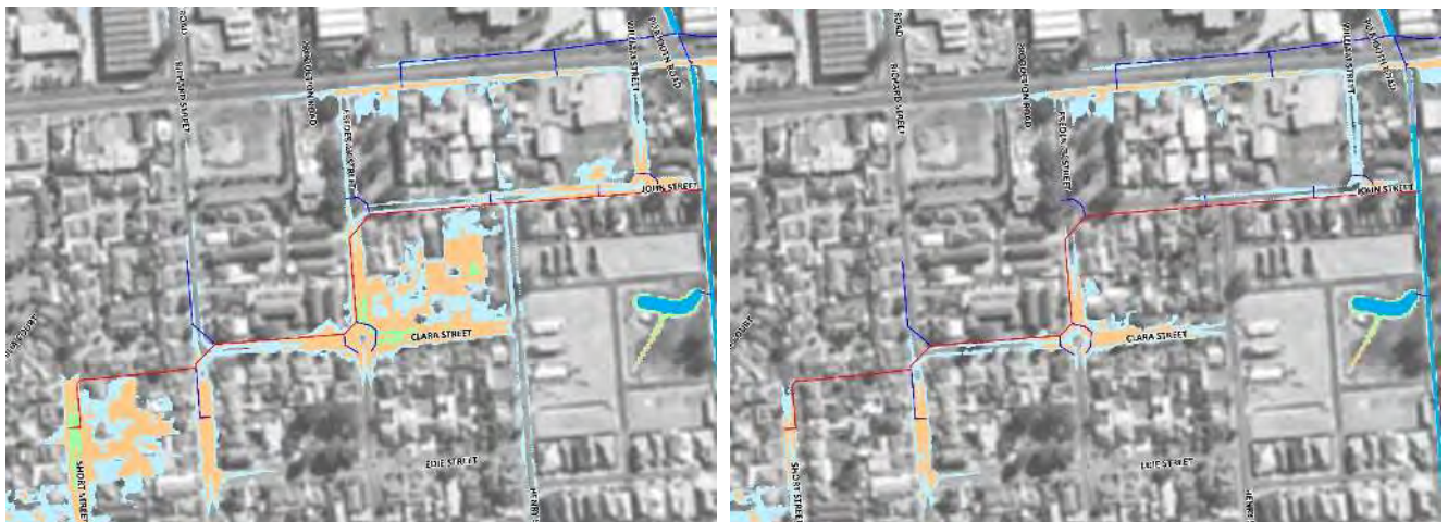
Figure 4.13 – D5 Stormwater Upgrade, 1% AEP Flood Maps, before (left) and after (right)
