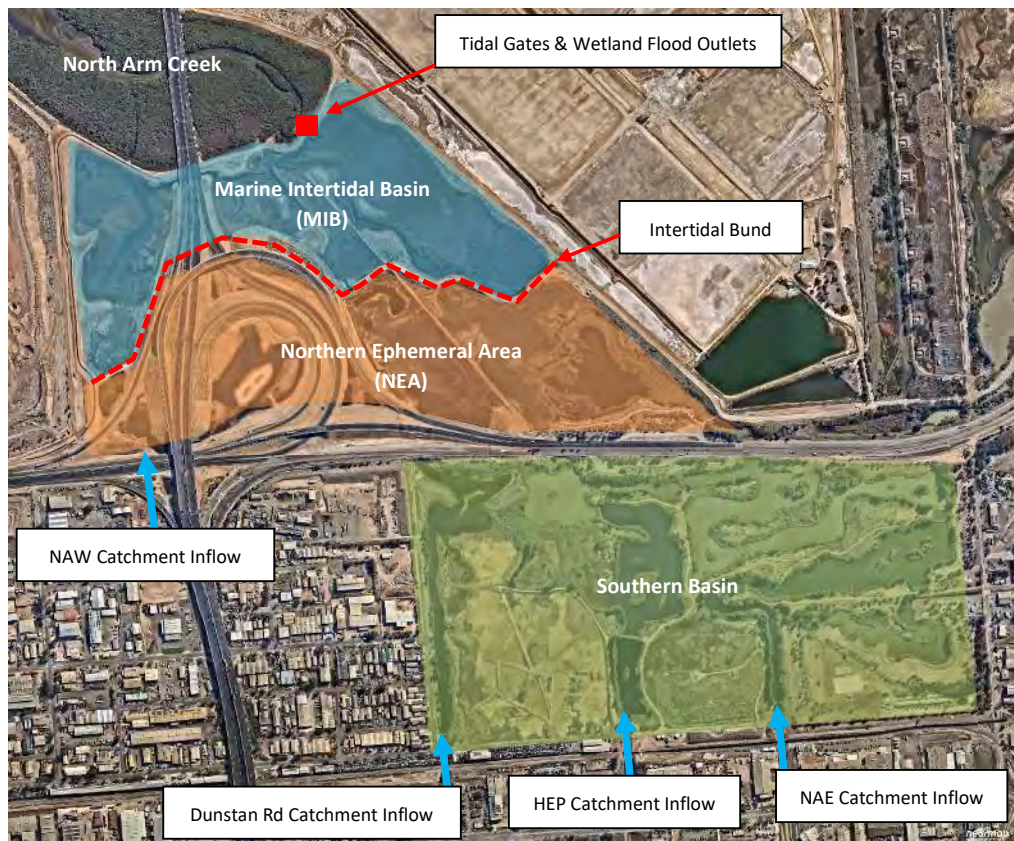
Figure 2.5 – Barker Inlet Wetlands Layout (Post Northern Connector Construction)
